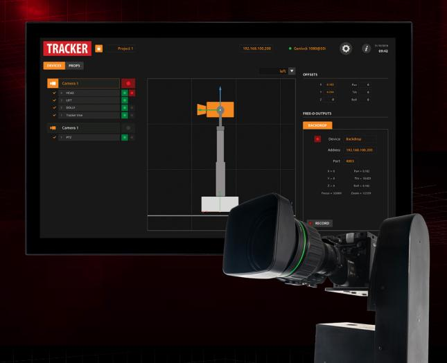
multiCAM TRACKER is an intuitive interface that compiles tracking data from different SPIRIT robotics to **generate a single FreeD signal per camera for virtual production engines**.
